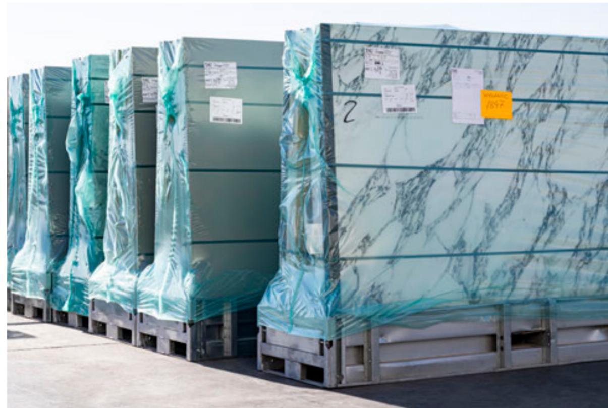
Trestles with ASCALE slabs must be loaded, unloaded and moved using a proper lift truck, crane or other handling mechanism.
