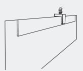
The additional width of this clamp will prevent the slab from bending during handling to, thus, prevent undesirable breakage.
